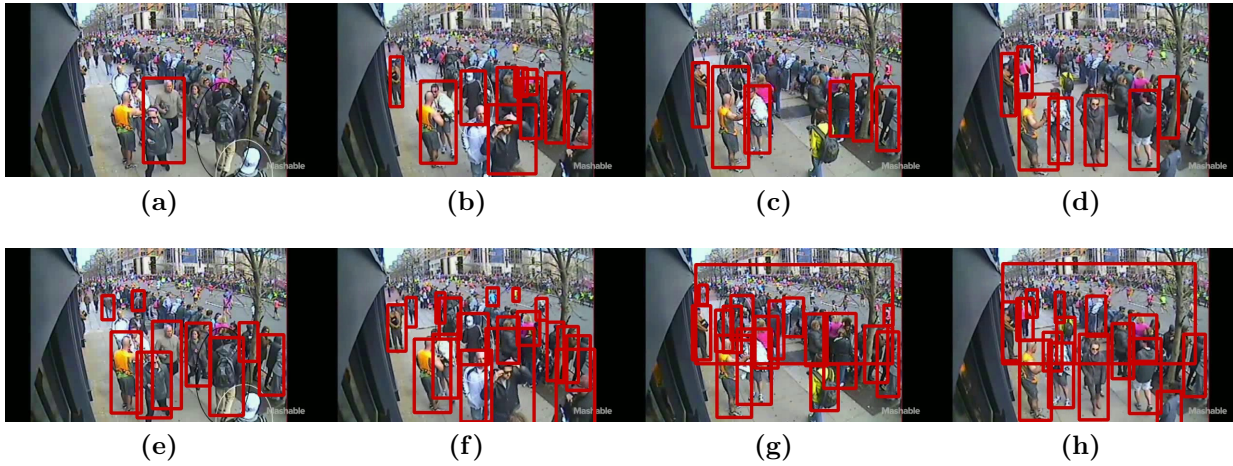
Figure 3.10: One artifact of the network at a low confidence threshold is the tendency to mislabel the entire crowd as one person. (tiny a-d, normal e-h)
